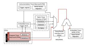
Fig. 3: CoreSight components in Xilinx Zynq
